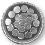
Before compression, a typical cross section of cable and lug consists of about 75% metal and 25% air.
